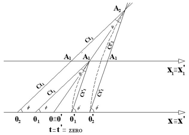
In the figure the angles have a relation  $\psi = \phi' - \phi$  and are equal to the following segments:
